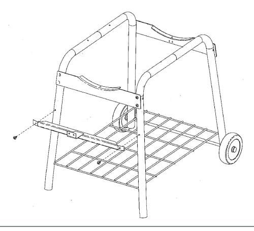
Install grill base (item #9), with firebox opening towards left side, on top of the legs using four M6 x 15mm Phillips head bolts. Install two M6 x 15mm Phillips head bolts and M6 hex nuts through grill base (item #9) and flange on leg braces (item #7)..
